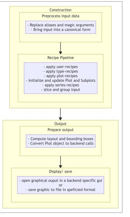
Figure 2 Plotting pipeline in Plots.jl. The separation of construction and output production enables the flexible use of different backends in the same session and helps to avoid unnecessary intermediate calculation. Created using mermaid [1].
