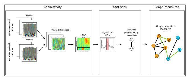
Figure 1 Schematic drawing of the three software parts: connectivity, statistics and graph measures.
