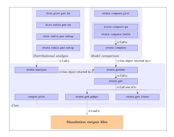
**Figure 1:** SimOutUtils architecture. Larger blocks with rounded corners and dashed outline constitute function groups, identified in italic font at the lower left corner of the respective block. Within these, functions are represented by smaller blocks with solid outline and sharp corners, with the function name shown in typewriter font. Arrows reflect the relationship between functions and between functions and function groups.
