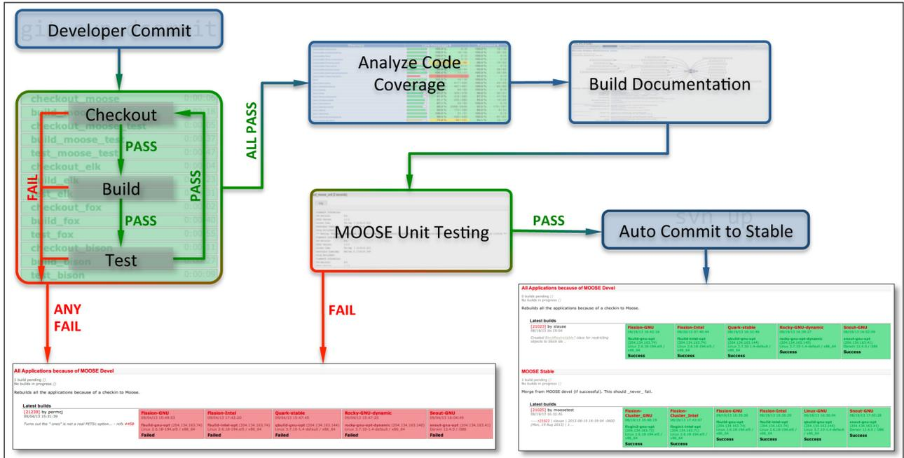
**Figure 1:** Flowchart depicting the MOOSE project's automatic build and testing system. After a developer commits a change, MOOSE and all the applications are built and tested. If any test fails, the system exits and reports failure. Otherwise, once all tests have succeeded, “stable” MOOSE is automatically updated, making it available to users.
