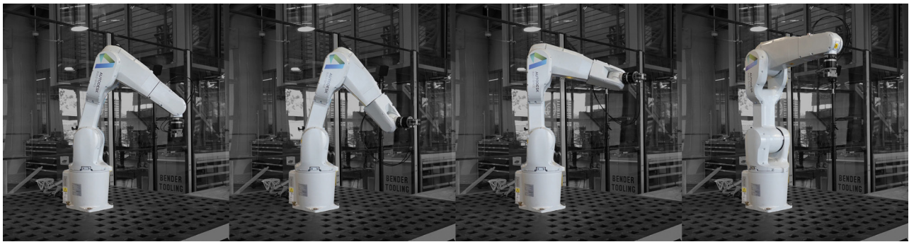
Figure 1: The four main motion actions of the Hello Robot program (Code Sample 1) executed on an ABB IRB 1200 robot—MoveTo(400, 300, 500), Rotate(0, 1, 0, -90), Move(0, 0, 250) and AxesTo(0, 0, 0, 0, 90, 0).
