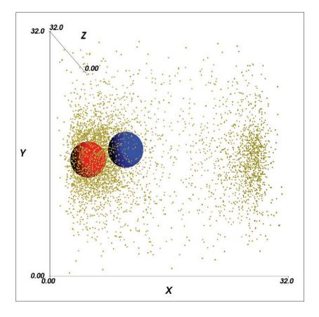
Figure 3: Output of the program view\_last\_simulation\_frame.py for the single dimer simulation with option --show-B. The product of reaction B is mostly found around the catalytic sphere (red) and the periodic character of the simulation box is visible.
